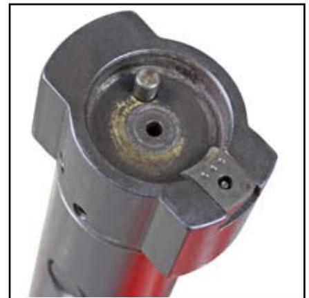
*The ArmaLite's bolt features dual front locking lugs and a massive extractor.*
