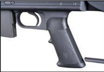
**The AR-30M features a detachable buttstock assembly that does not tie to the M16-type synthetic pistol grip.**
